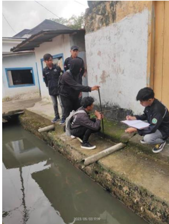
Figure 3.2 Measuring Channel Width
